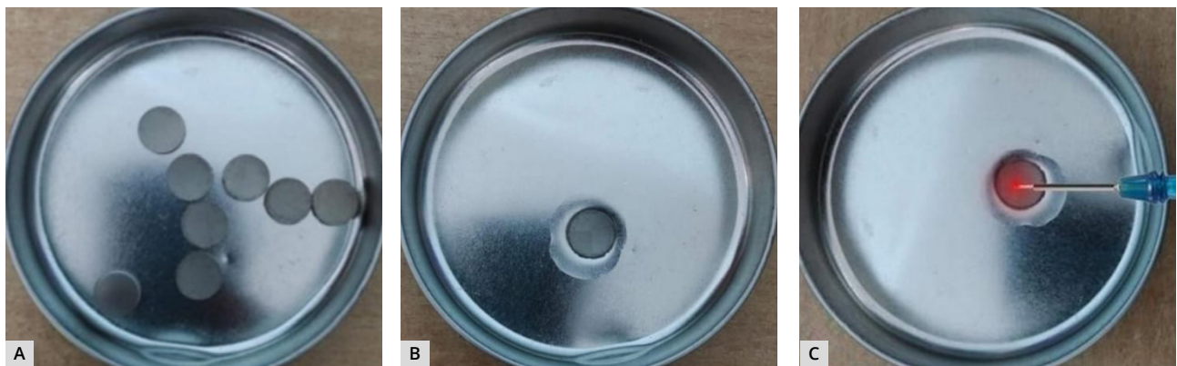
Figure 2. A) Titanium discs. B) Discs with test material. C) Discs with laser treatment.
